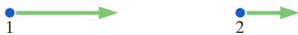
Figure 1.7 Two successive positions of a particle (indicated by a dot), with arrows indicating the velocity of the particle at each location. The shorter arrow indicates that the speed of the particle at location 2 is less than its speed at location 1.
