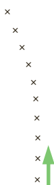
Figure 1.5 A proton moves through space, far from almost all other objects. The initial direction of the proton's motion is upward, as indicated by the arrow. The \times 's represent the position of the proton at equal time intervals.
